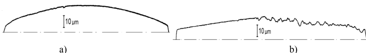
Fig. 3. Profiles of ring face: first compression one (a) and second compression one (b)
